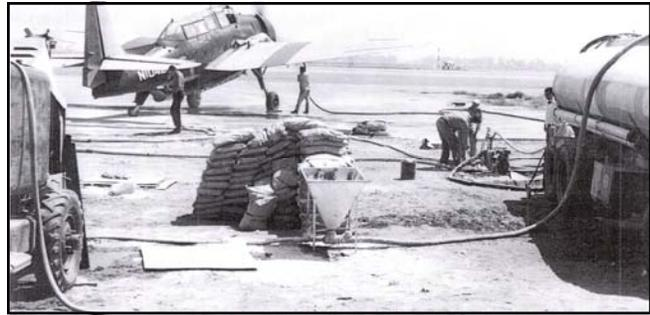
**TBM Air Tanker (USFS owned) and Borate Mixing / Loading System, Ontario, CA, 1957**
